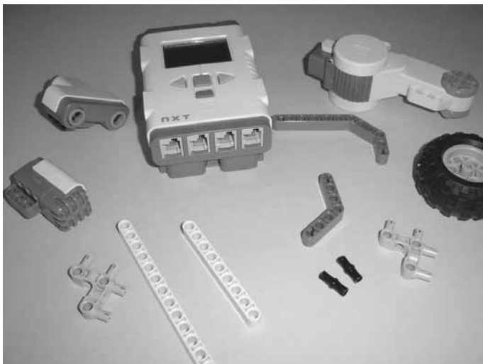
Figure 1-3. Mindstorms NXT Intelligent Brick and other components
